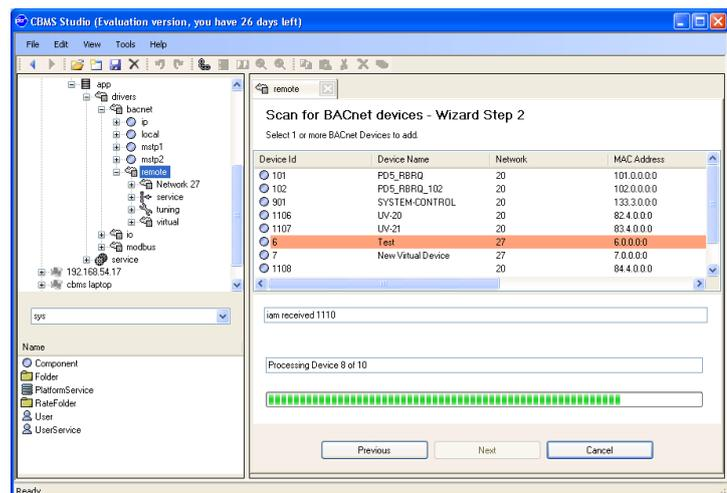
The BACnet objects are located in a folder called virtual beneath the device object. When an object is selected it's properties can be viewed from the BACnet property sheet. Any property that is writable can be updated from the property sheet.
